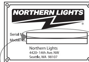
Generator Set Serial Number
